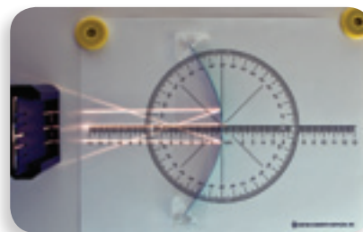
Mirror can be adjusted to demonstrate concave (shown) and convex properties.
