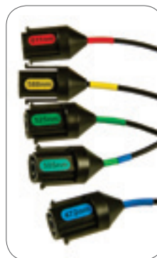
Each of the five LEDs carries an identifying color band and a color patch with the wavelength maximum.
