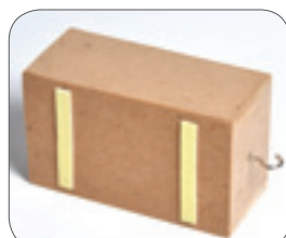
Two leather strips are attached to the bottom of the Friction Box.
