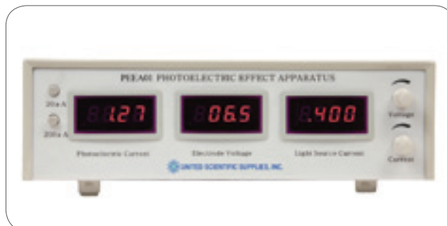
The control and measurement unit contains a highly stabilized lamp power supply adjusted by a multi-turn potentiometer.
