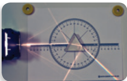
Light box and prism are used together to produce a spectrum.
